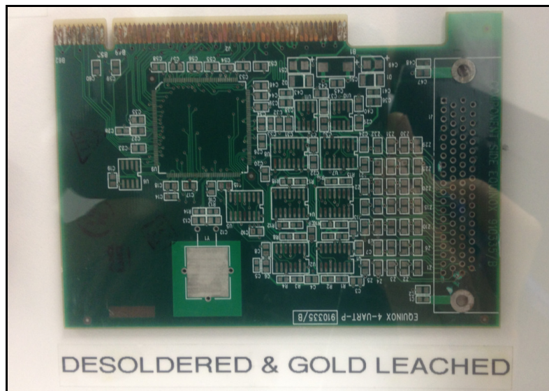
Figure 5. Desoldered and Gold Leached Printed Wiring Board
